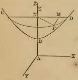
verse axis. Let CBD be an hyperbola, and let it be revolved about its transverse axis BE; then any point on the curve, as D, in its revolution will describe the circumference of a circle. Let the origin be placed at the centre of the hyperbola, and let the transverse axis of the hyperbola be the axis of z.
